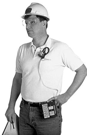
Clip holder to worker and pump to belt.
