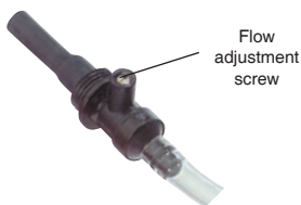
Calibration train with tube in low flow holder
