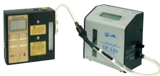
Calibration train with tube in low flow holder
