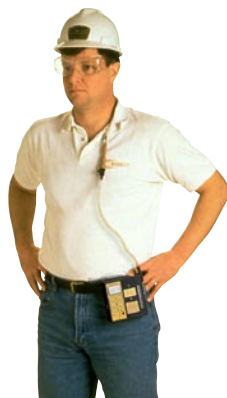
Clip holder to worker and pump to belt.
